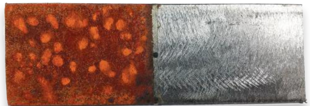
3/16" inch thick bare steel. Right side brushed with Rust Pro and wiped off. Steel exposed to open air (67°F, 63% humidity) and muriatic acid for 24 hours.
