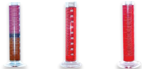
FUEL STORAGE TANKS # 2 DIESEL 95 ML TREATED WITH FUEL MAXIMIZER 58% WATER REMOVED 42% EMULSIFIED 94 ML
